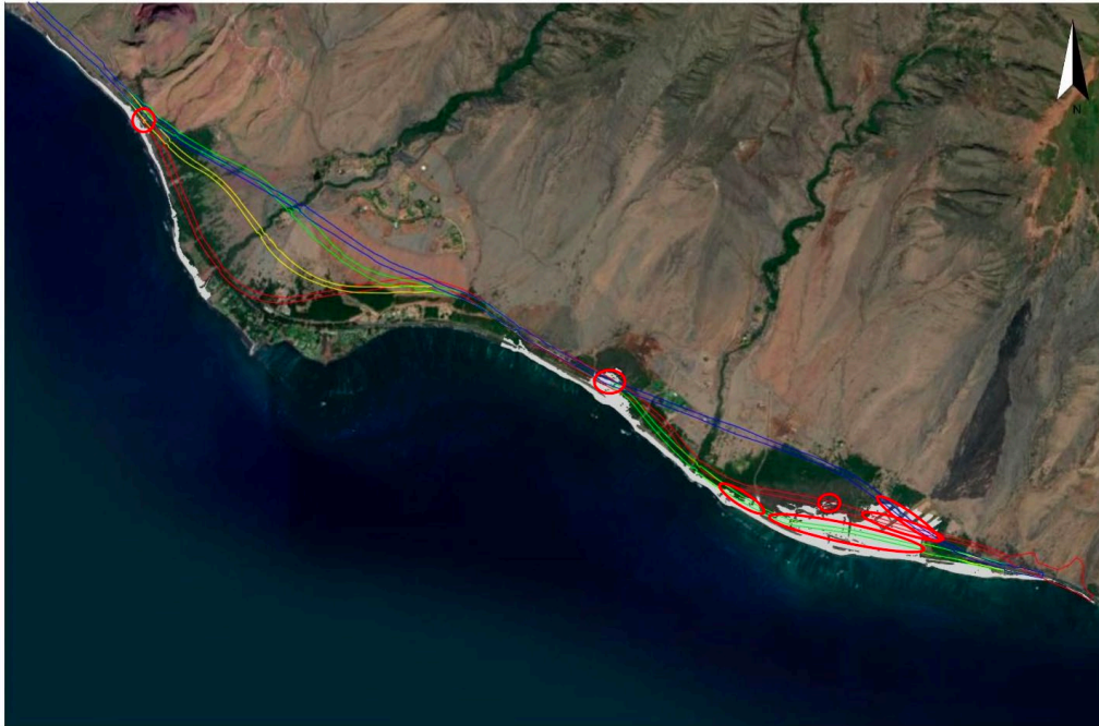
Figure 5-5. XBeach-NH modeled maximum flood extent (gray) for existing ground relative to alternatives 1 (red), 2 (yellow/green), 3 (green), and 4 (blue) alignments. Overlapping flooded areas are outlined in red.
