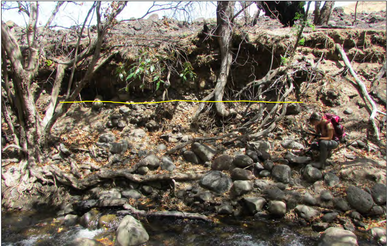
Photo 85. OHWM Level in the Middle Reach of the Stream in Study Area Below the Soil Erosion Seen on Top of the Bank
