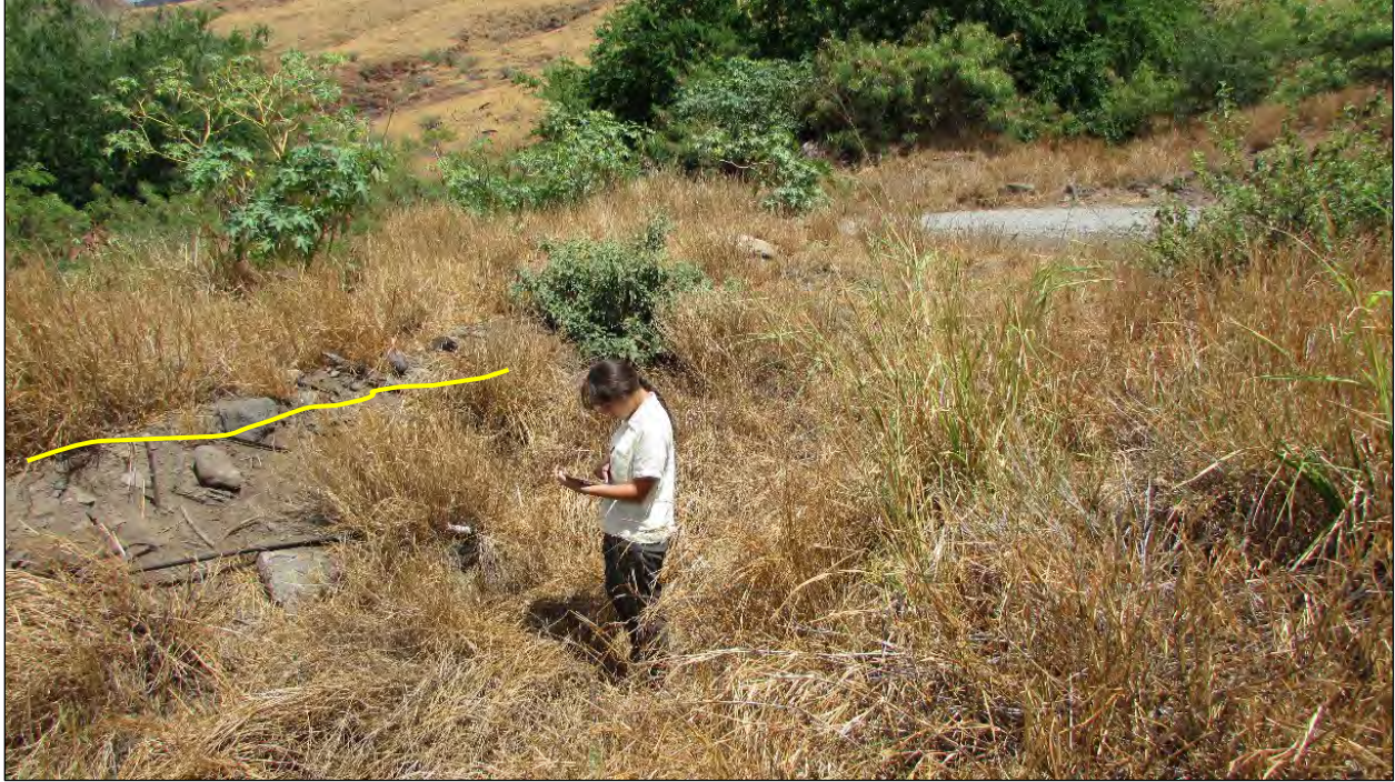
Photo 88. Location of Transect 1; Representative of the Uppermost Reach of the Stream in the Study Area (Break in Slope and Washed of Debris Were Used as Indicators of OHWM)
