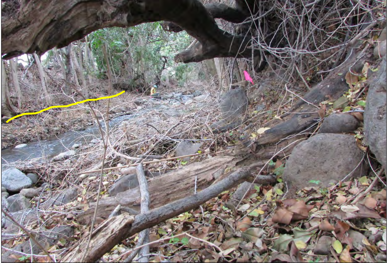
Photo 71. Location of Transect 2 in Middle Reach of Stream; Transect Placed Where Clear Lining on the Bank was Visible at the OHWM Level Along with Sediment Sorting from Boulders to Sediment
