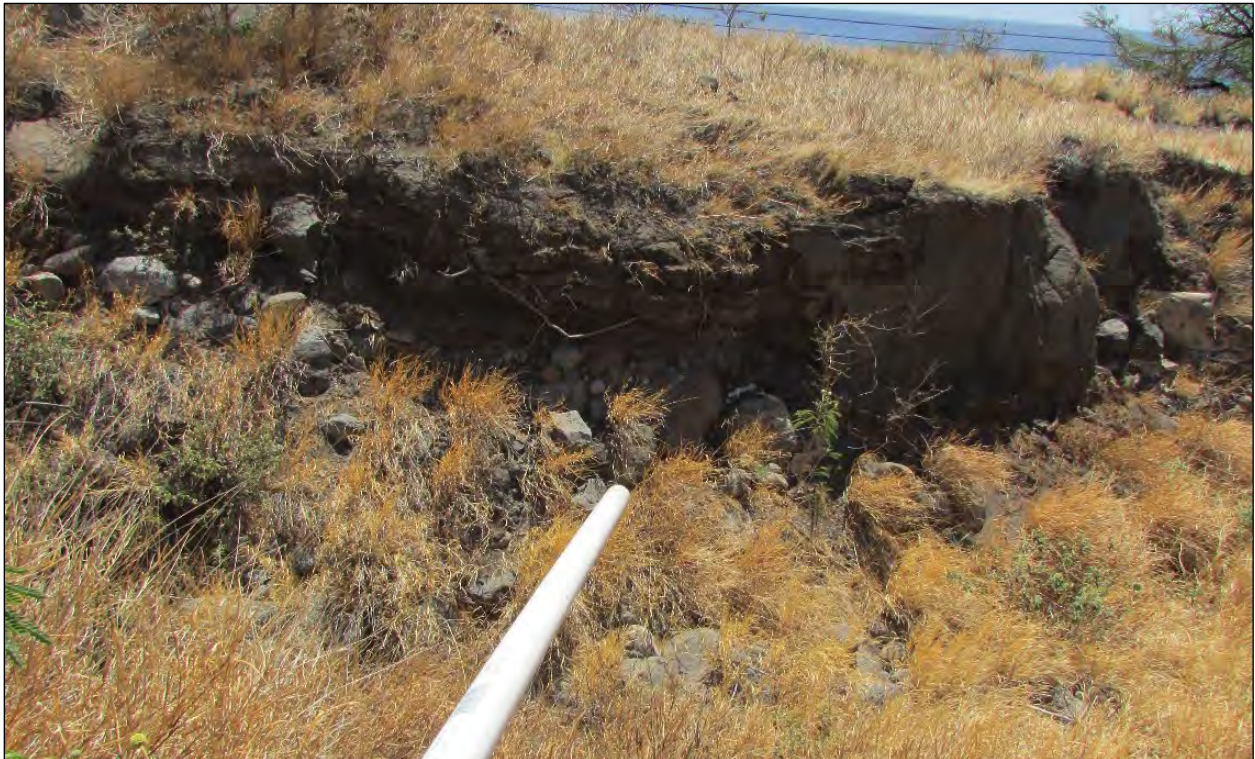
Photo 95. Awalua Stream Undercut Bank; Vegetation Line Together with Undercut Bank Allowed for Identifying OHWM Level Here
