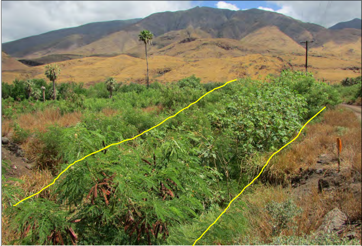
Photo 90. Location of Transect 2 at the Lower/Western Reach of Lihau Stream in the Study Area; Heavily Vegetated Moist Bed Compared to the Upper Drier Banks and Break in Bank Slope Used as OHWM Indicators
